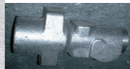
Original machining methods OD chucking with Tailstock support => OD and Flange both facing.
